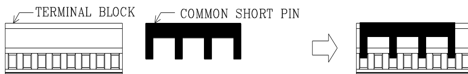
Terminal Block and Common Shorting Pin Assembly
